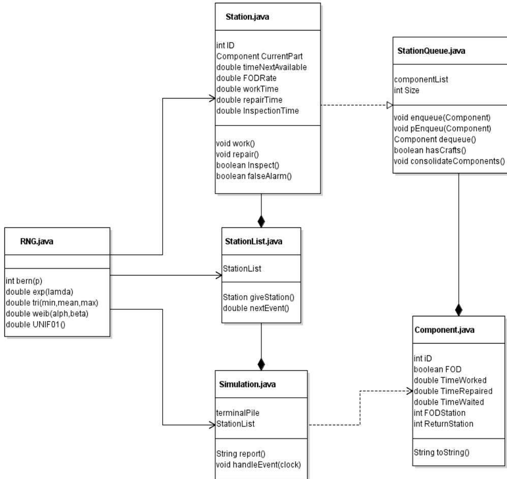
Figure 26: Simulation UML Diagram
