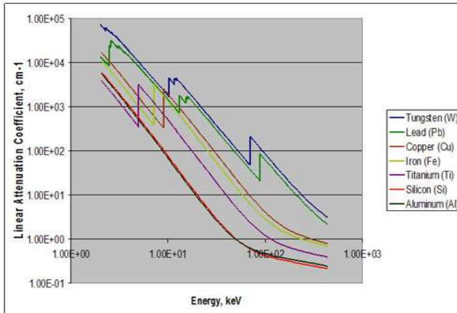
Figure 21: Linear Attenuation Coefficient vs Energy
