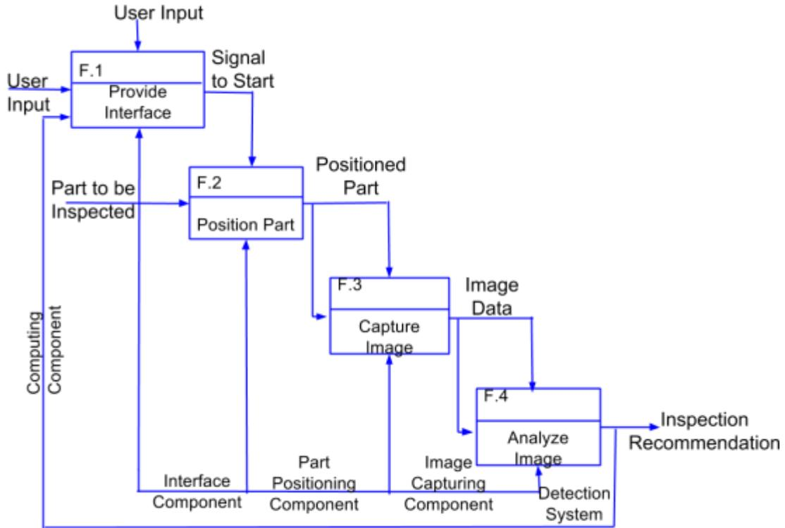
Figure 11: IDEF.0 for Enhanced Inspection System
