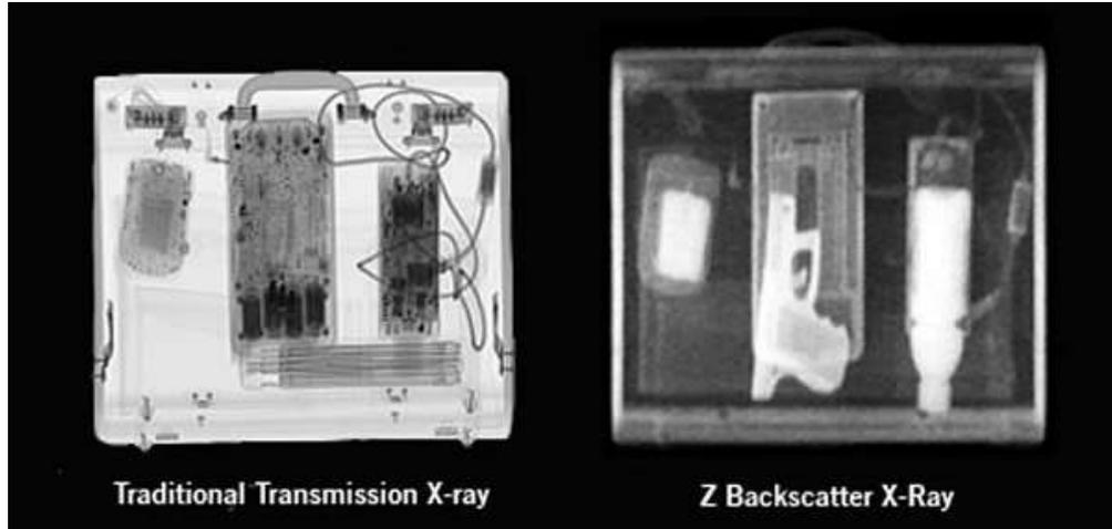
Figure 14: Traditional Transmission X-ray Vs Z Backscatter X-Ray
