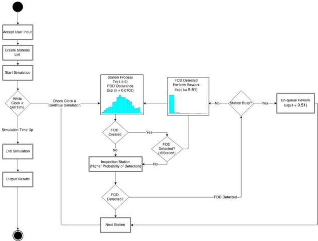
Figure 27: Simulation Flow Diagram
