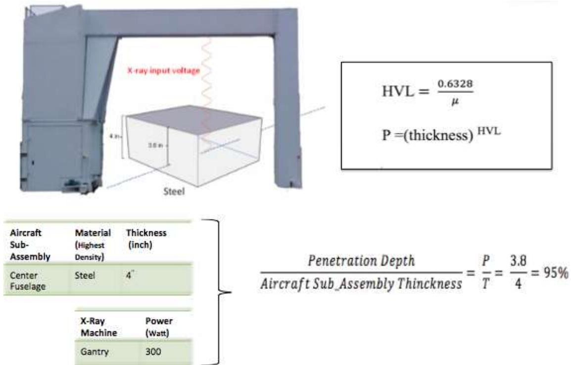
Figure 18: Penetration Depth Example
