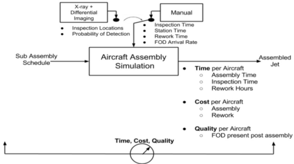
Figure 25: Aircraft Assembly Simulation Diagram
