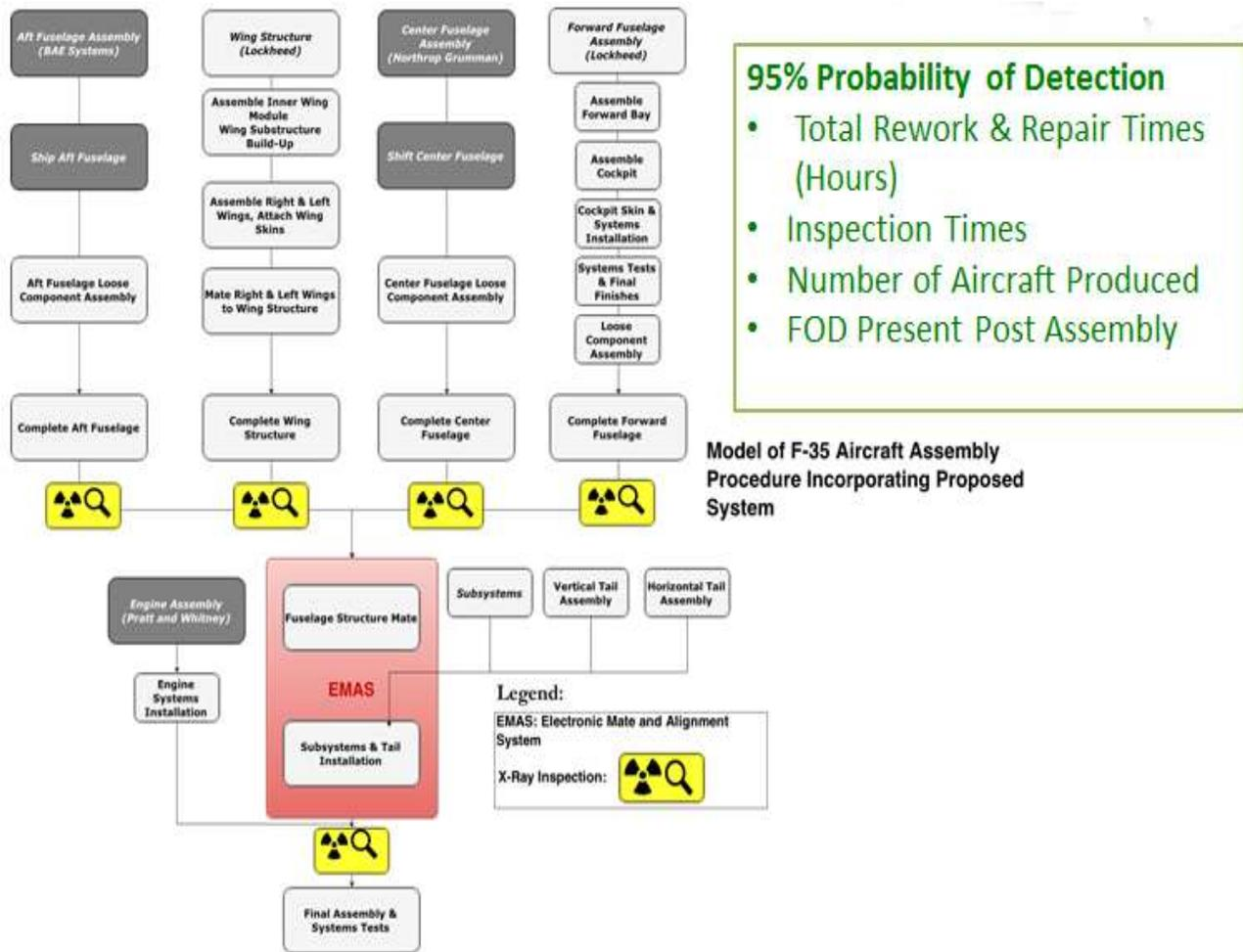
Figure 7: Aircraft assembly flow with Enhanced Inspection
