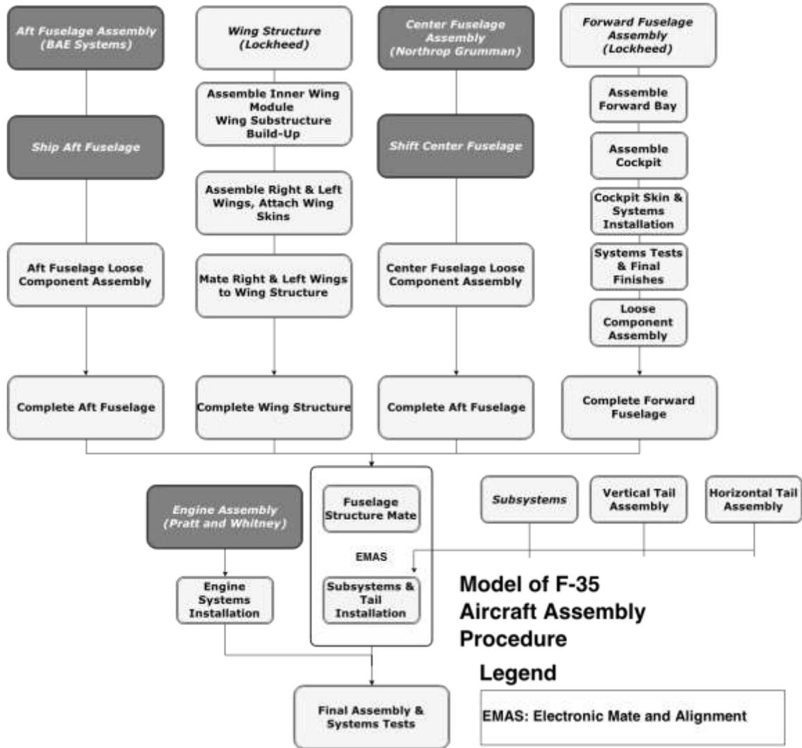
Figure 1: Aircraft Assembly Flow
