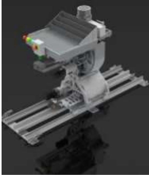
The linear rail is an adjustable system; the length can be adjusted based on the desired object being scanned or can be adjusted to image different lengths/portions of the object. The linear Search system is designed in a way to scan objects either straight up or upside down. The system is set up in a way to move requiring 2 people (MiGFlug).
