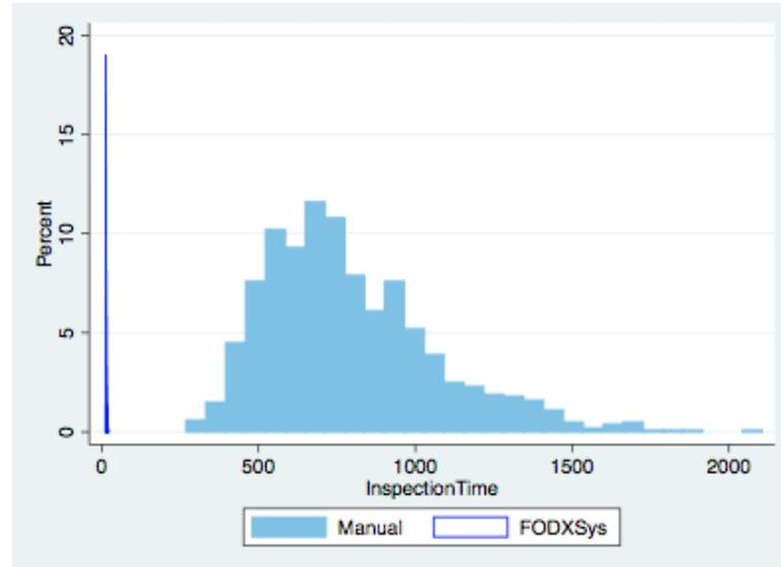
Figure 29: Inspection Time Distribution (Manual vs FODXSYS)
