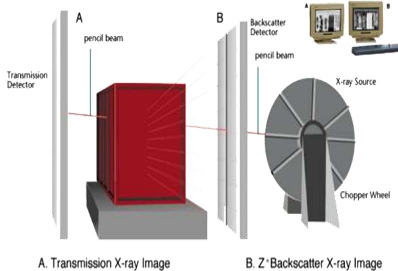
Figure 13: Transmission vs Backscatter
