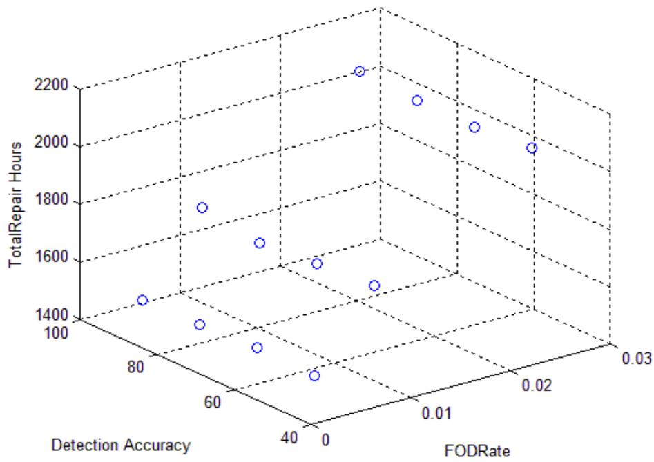
Figure 35: Detection Accuracy vs FOD Rate vs Total Repair Hours
