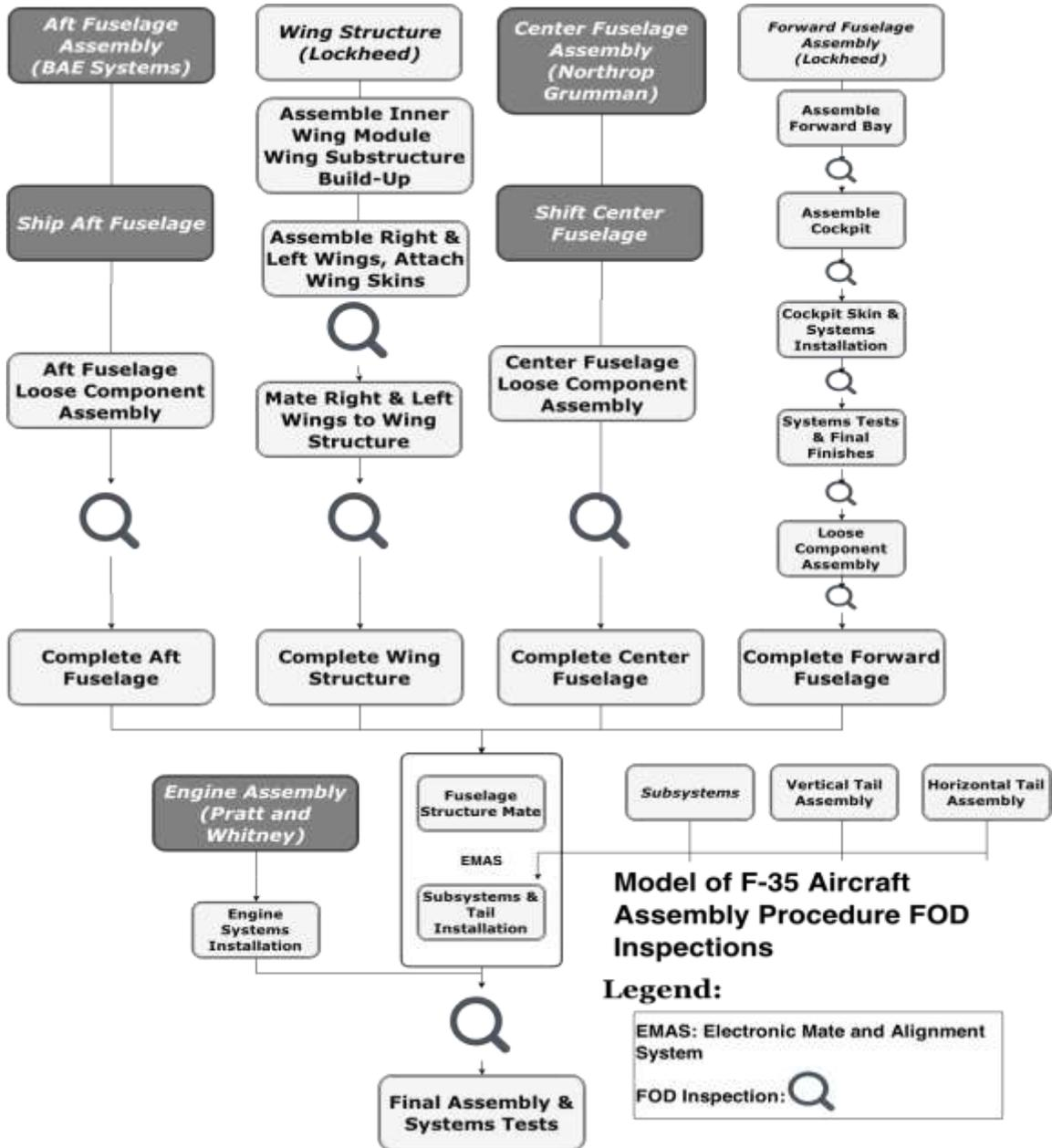
Figure 2: Aircraft assembly flow with Manual Inspection
