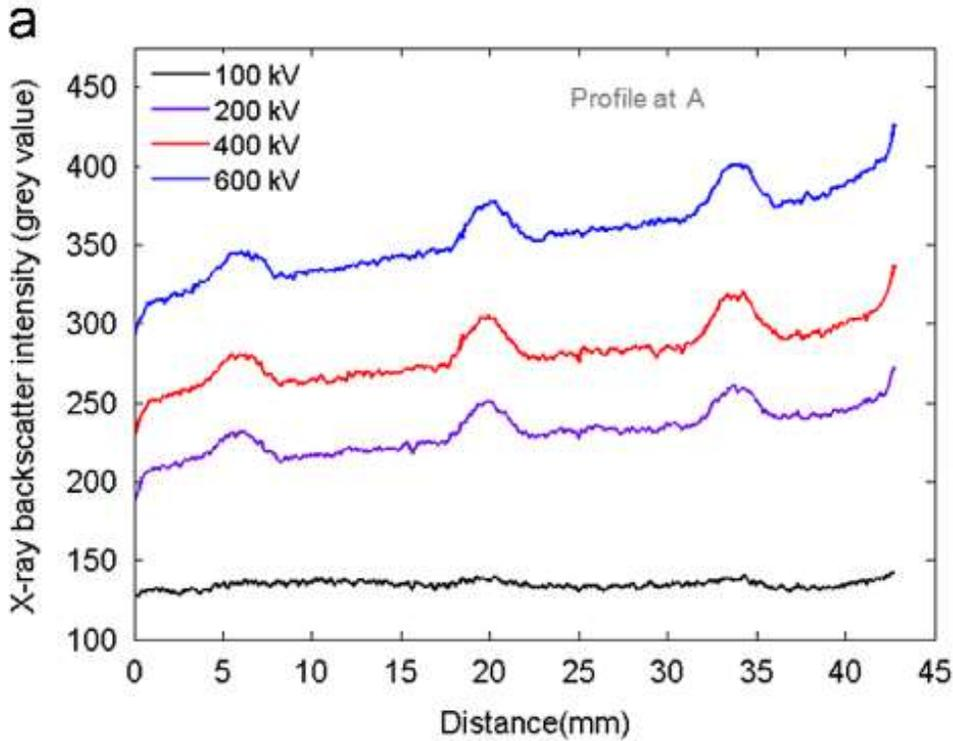
Figure 20: Intensity based on Varied Input Voltage
