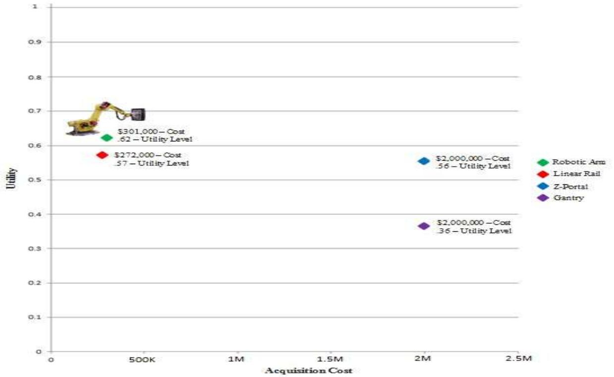
Figure 23: X-ray Mounting Alternatives Utility vs Cost
