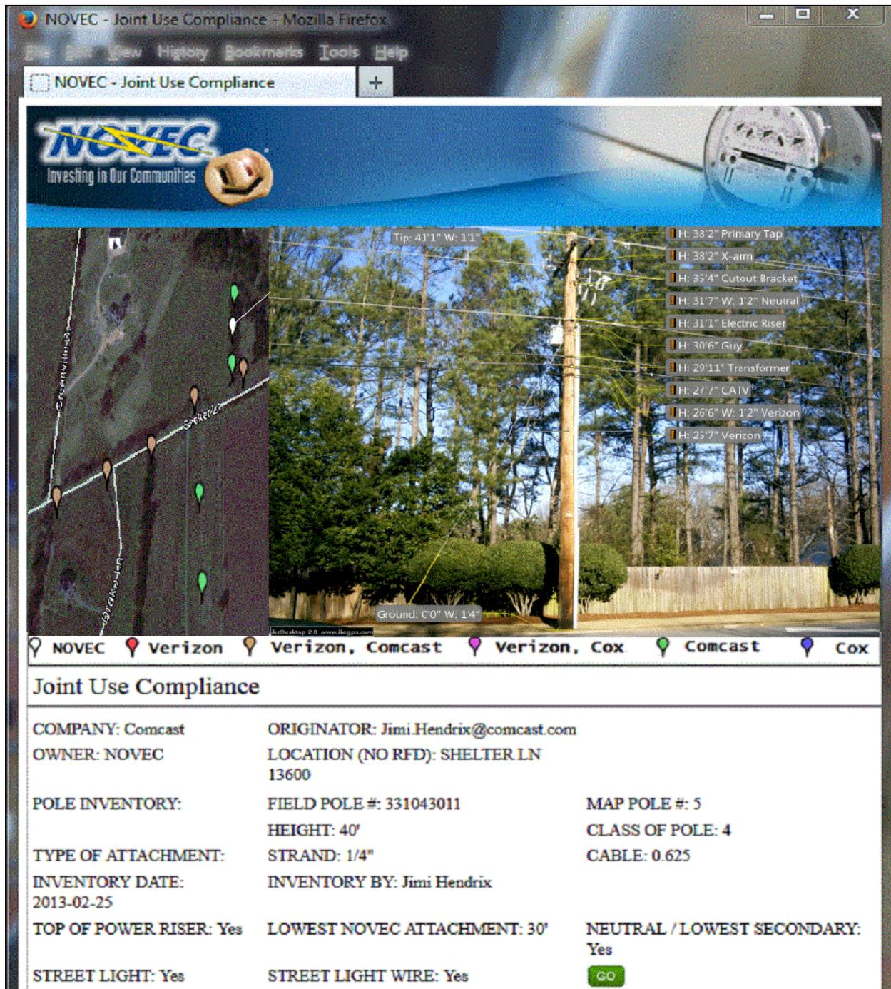
Figure 22: 3rd Party Attachment Compliance Prototype
