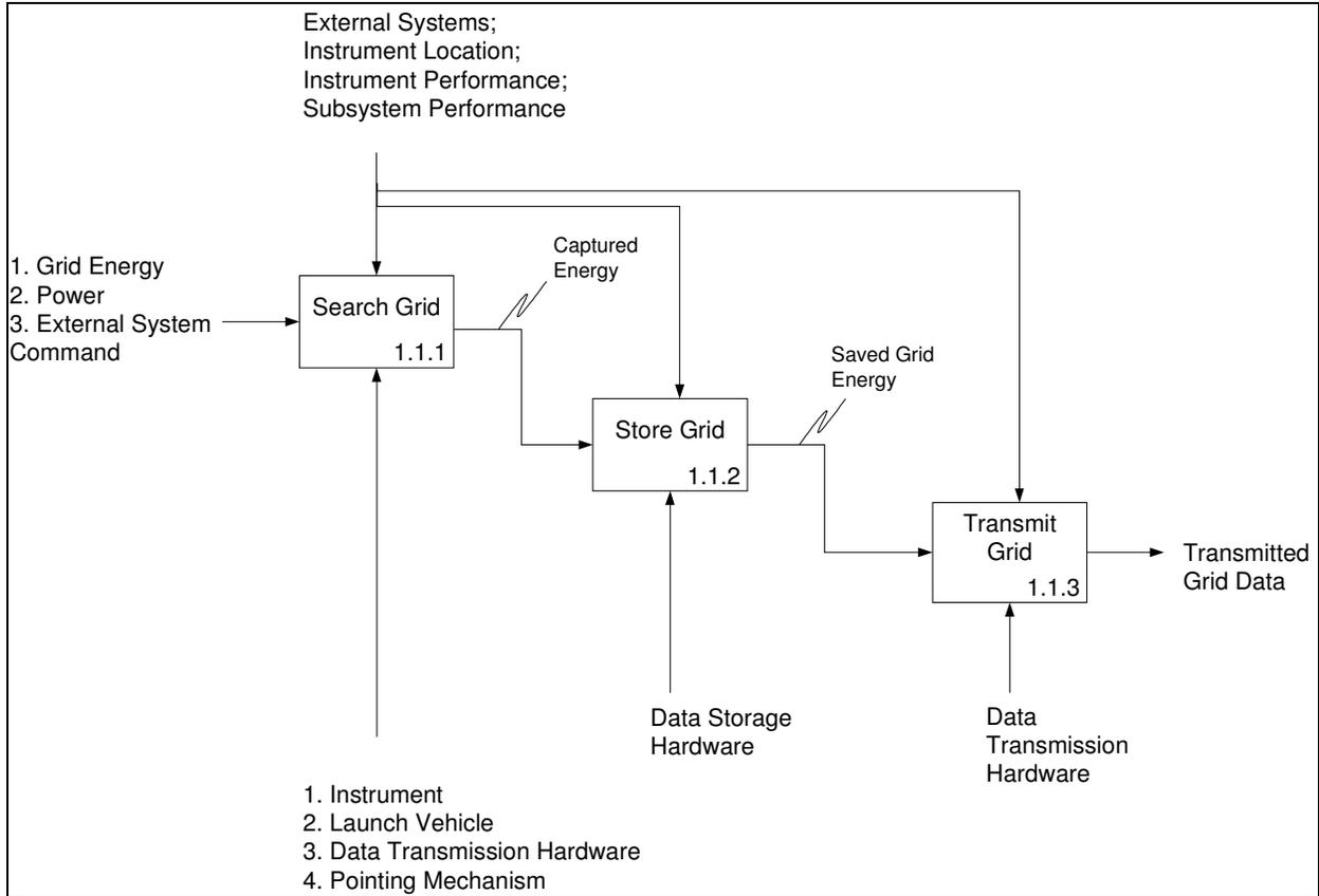
**Figure 30: Level 2 Functional Architecture**
