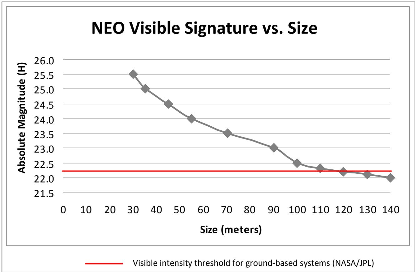
**Figure 3: Limiting Magnitude of Current Ground-Based NEO Observation Systems (NASA)**
