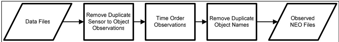
Figure 9: SNOOS Initial Post Processing Steps
