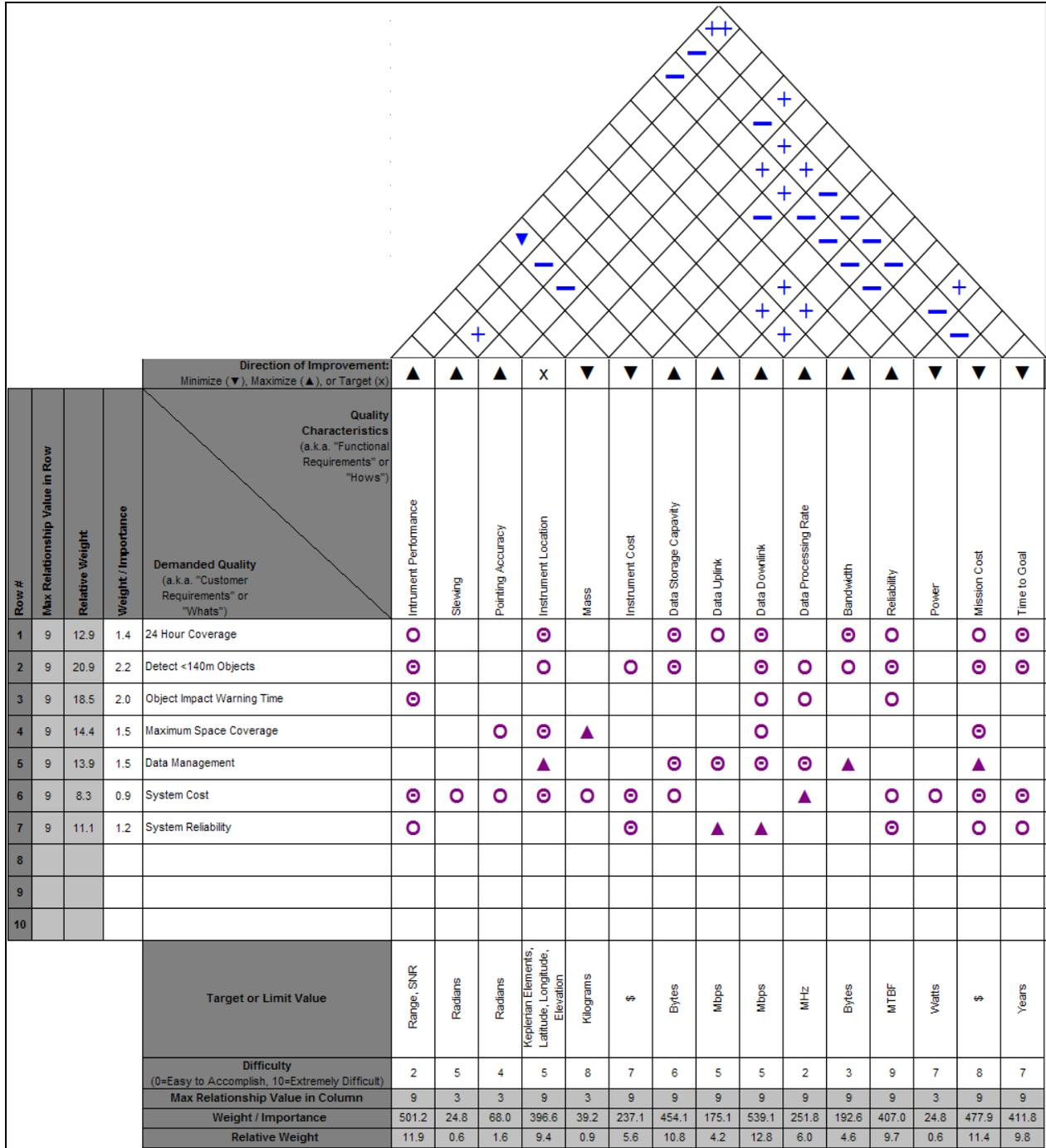
Figure 23: SNOOS Quality Function Deployment Matrix
