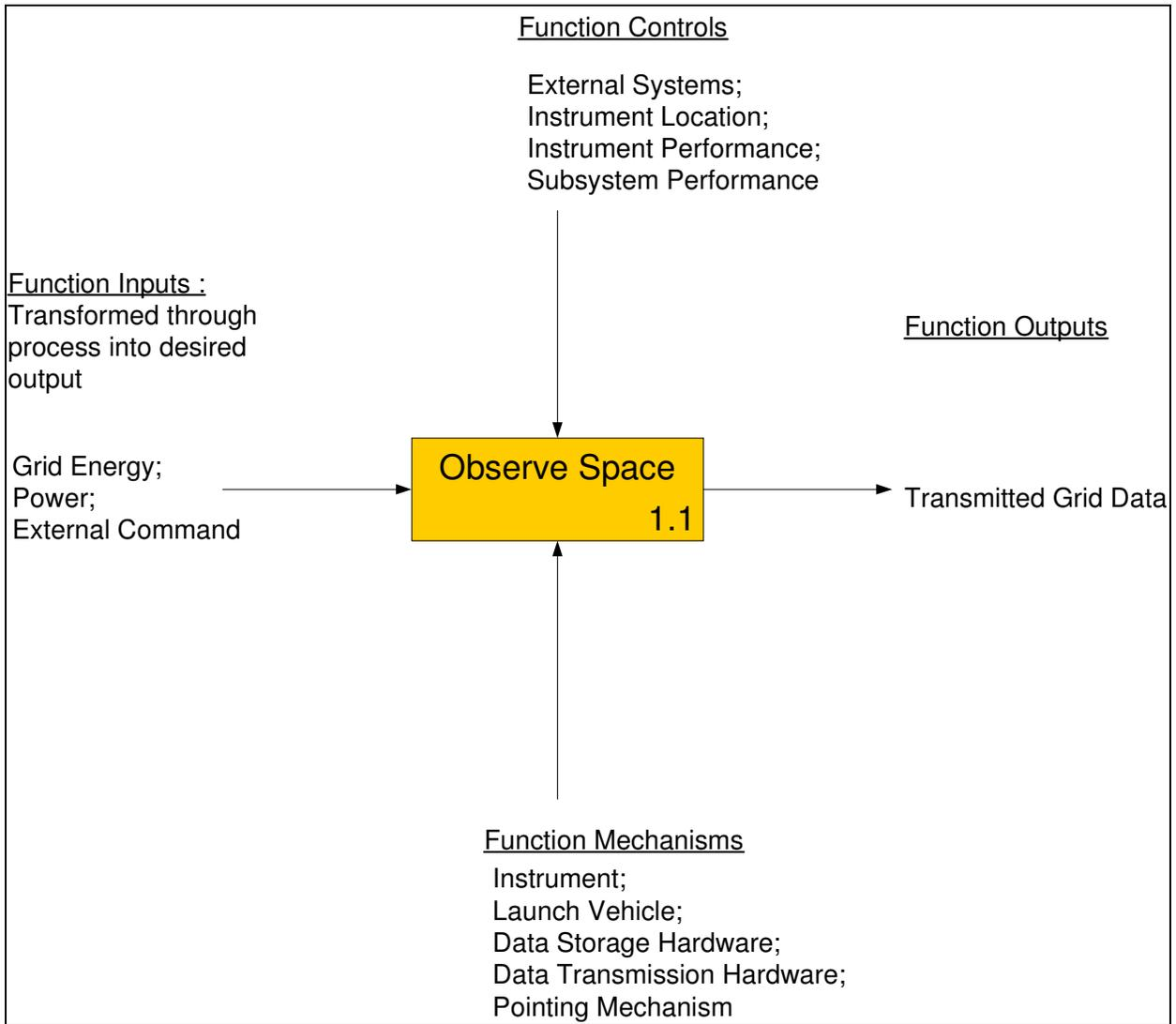
Figure 29: Level 1 Functional Architecture
