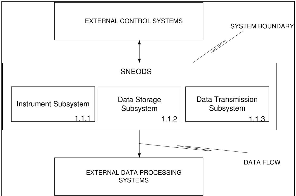
Figure 27: External Systems Diagram
